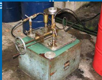
Deadweight tester in the valve chamber.
